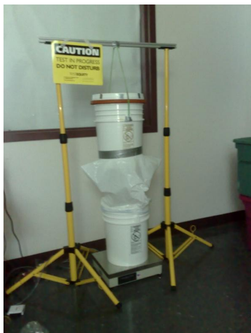
Figure 5 Model experimental setup for flow experiments conducted for different filter variants.
